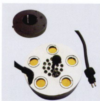
ITEM NO. : 05B DIAMETER:Φ100MM H: 33MM WATERLEVELSENSORSWTCH:H35MM POWER:DC 36V 140W FOG VOLUME:1500ML/H
