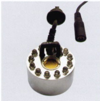
ITEM NO. : 01A DIAMETER: Φ45MM H: 38MM INPUT VOLTAGE: A/C 24V 28W FOG VOLUME: 90-300ML/H CERAMIC DIA: 16MM 12 LAMPS
