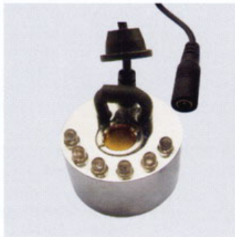
ITEM NO. : 01F DIAMETER: Φ38MM H: 44MM INPUT VOLTAGE: A/C 24V 26W FOG VOLUME: 90-300ML/H CERAMIC DIA: 16MM 6 LAMPS
