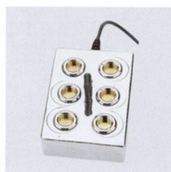
ITEM NO. : AT-06 MIST MAKER:153*88*27MM WATERLEVELSENSORSWTCH:H25MM POWER:DC 48V 140W FOG VOLUME:1800ML/H
