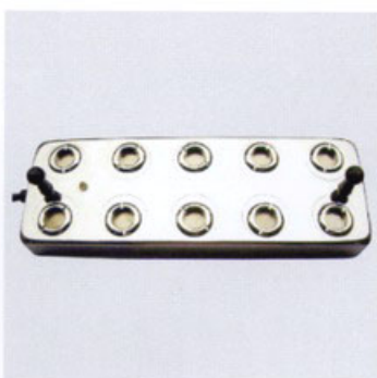
ITEM NO. : AT-010 WATERLEVELSENSORSWTCH:H26MM POWER:DC 48V 225W FOG VOLUME:3000ML/H CERAMIC DIA:20MM
